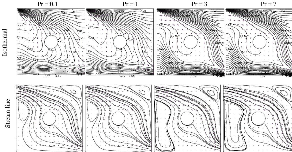
Fig. 6. Isotherms and Streamlines for the TB configuration at different Pr While  $dr = 1.0$ ,  $Ri = 1.0$  and  $L_x = L_y = 0.5$ .
