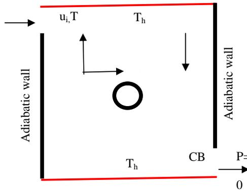
Fig. 1. Schematic diagram of the square cavity.
