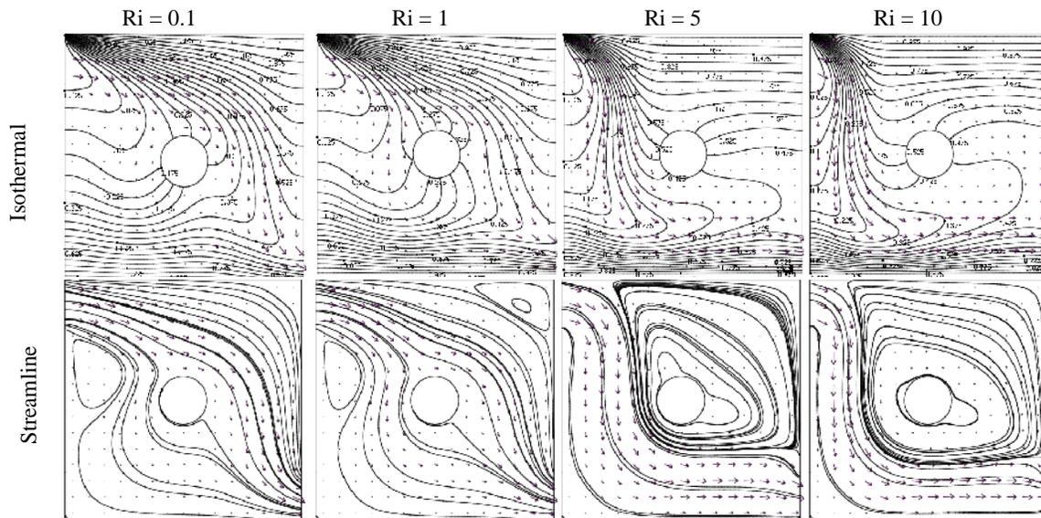
**Fig. 5.** Isotherms and Streamlines for the TB configuration at different diameter ratio ( $dr$ ) While  $Re = 100$ ,  $Ri = 1.0$  and  $L_x = L_y = 0.5$ .
