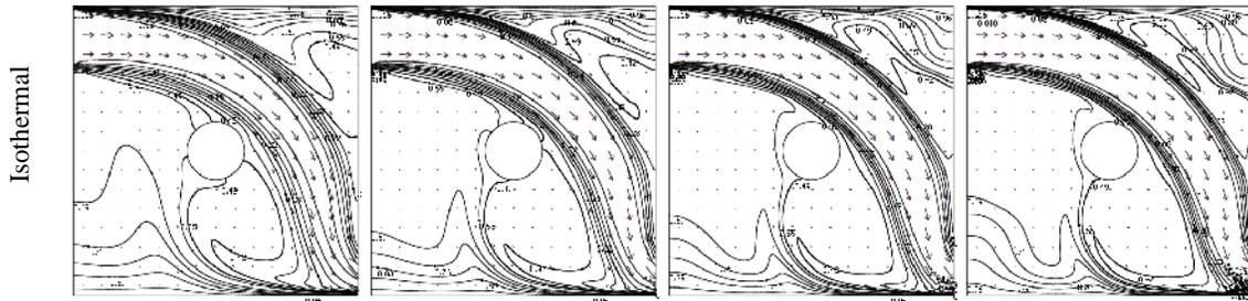
**Fig. 4.** Isotherms and Streamlines for the TB configuration at different Re While  $dr = 1.0$ ,  $Ri = 1.0$  and  $L_x = L_y = 0.5$ .
