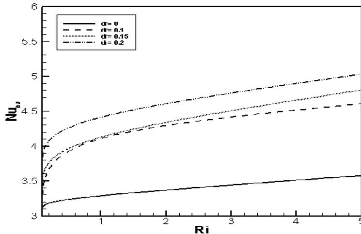
Fig. 7. Effect of cylinder diameter on  $Nu_{av}$  for the TB configuration While  $Re = 100$ ,  $Ri = 1.0$  and  $Pr = 0.71$ .
