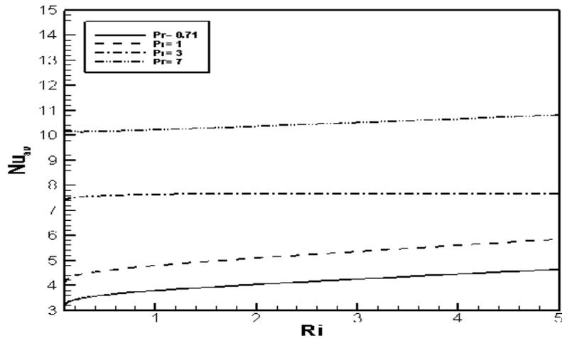
Fig. 8. Effect of  $Pr$  on  $Nu_{av}$  for the TB configuration While  $Re = 100$ ,  $Ri = 1.0$ .
