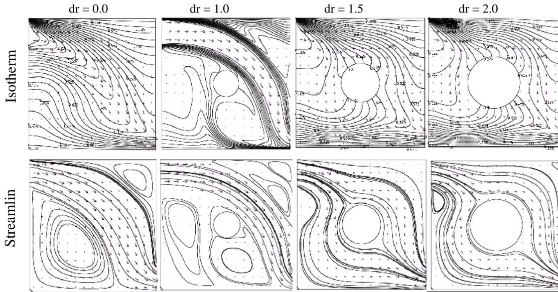
**Fig. 3.** Isotherms and Streamlines for the TB configuration at different diameter ratio ( $dr$ ) While  $Re = 100$ ,  $Ri = 1.0$  and  $L_x = L_y = 0.5$ .
