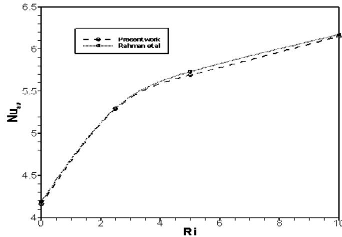
**Fig. 2.** Comparison of the average Nusselt number with the Richardson number while  $Re = 100$ ,  $Pr = 0.71$  and  $k = 10$ .
